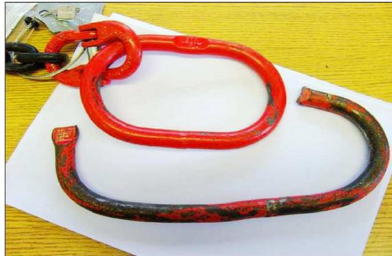
Significant deformation in left-hand corner of link (top)
